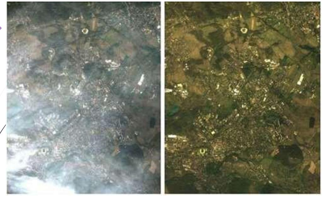
Figure 1.6: Atmospheric correction
