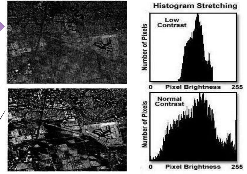
Figure 1.13: Contrast Enhancement by Histogram Stretch
